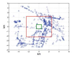
Figure 5: Two models of the distribution of base stations in Tokyo. Those generated by hexagonal grid method are represented as triangles and those generated by the Poisson point process method as diamonds. Again, 25% of the population lives in the red rectangle, 1% of the population in the smaller green rectangle. Source: [9].
